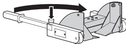
**Route cable so that it is not in contact with the grey parts shown in the drawing.**
