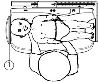
1. Place the baby on the weighing tray. The baby's head must be positioned at the head stop (1) of the tray.
